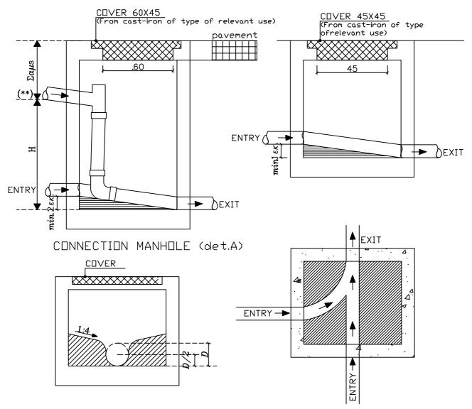
TYPICAL SECTION OF SEWER MANHOLE
